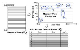
Fig. 6. Memory view clustering.  $R_X^6$  is a set of access control rules for an MPU that supports 6 protected memory regions at maximum.
