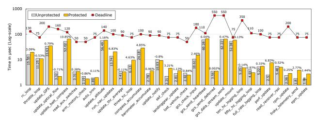
Fig. 8. Performance impact of MINION on real-time tasks with deadline constraints. The overhead introduced by MINION is marked on top of every bar that represents the execution time with MINION. The results are the average of more than 100 runs.
