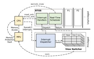
Fig. 7. Detailed architecture of memory view enforcement.
